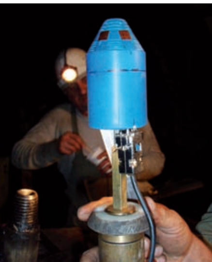
Conical probe for rock stress measurement constructed at the institute.
